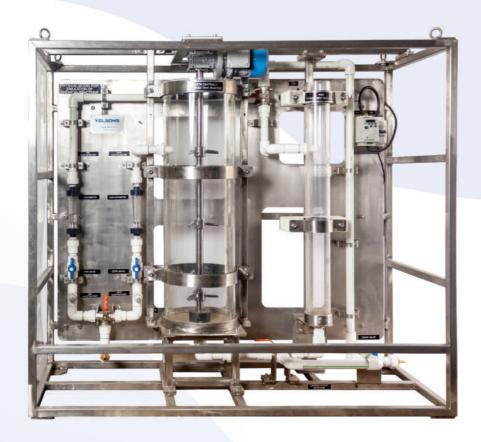
The flow rig / RTD simulator will be used to perform various permutations and combinations of flow rate, speed of the agitator and type of the vessel to understand flow dynamics in scaled down models of CSTR and column type reactors.
